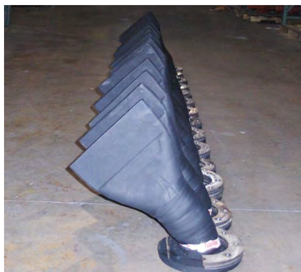
A 4" Tideflex Widebill Diffuser (left) next to a standard 4" Tideflex Diffuser (right).
